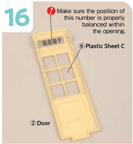
Peel off the double-sided tapes' backings, and affix ⑥ Plastic Sheet C of step 14 as shown.
